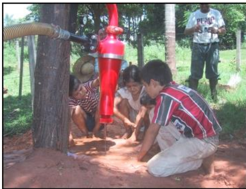
We also have a new sand cone Besides getting the sand out of the drilling mud, it provides lots of fun for the kids
